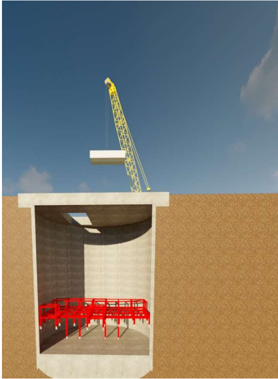
Installation of the shelter roof
